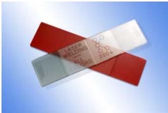
Fig. 7: Laser weld of two optically transparent plates resp. two two identically colored plates (lying underneath)
