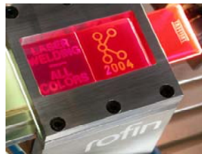
Laser weld of fluorescent plates (lower plate with Lumogen® IR)
