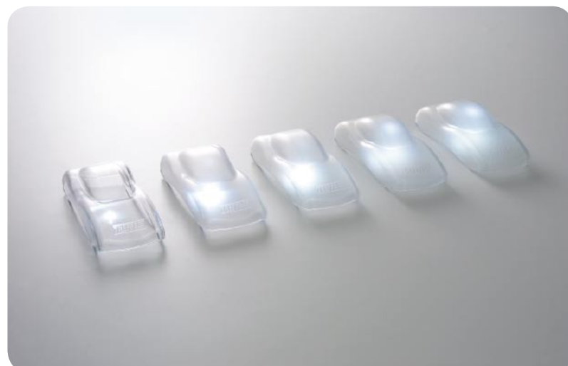
Fig. 4: an LED lighting and the effect with different concentrations of light diffusion additives
